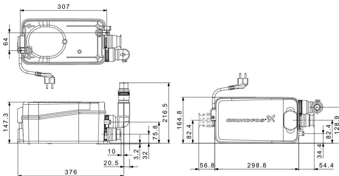
Fig. 44 Dimensions, Sololift2 D-2
