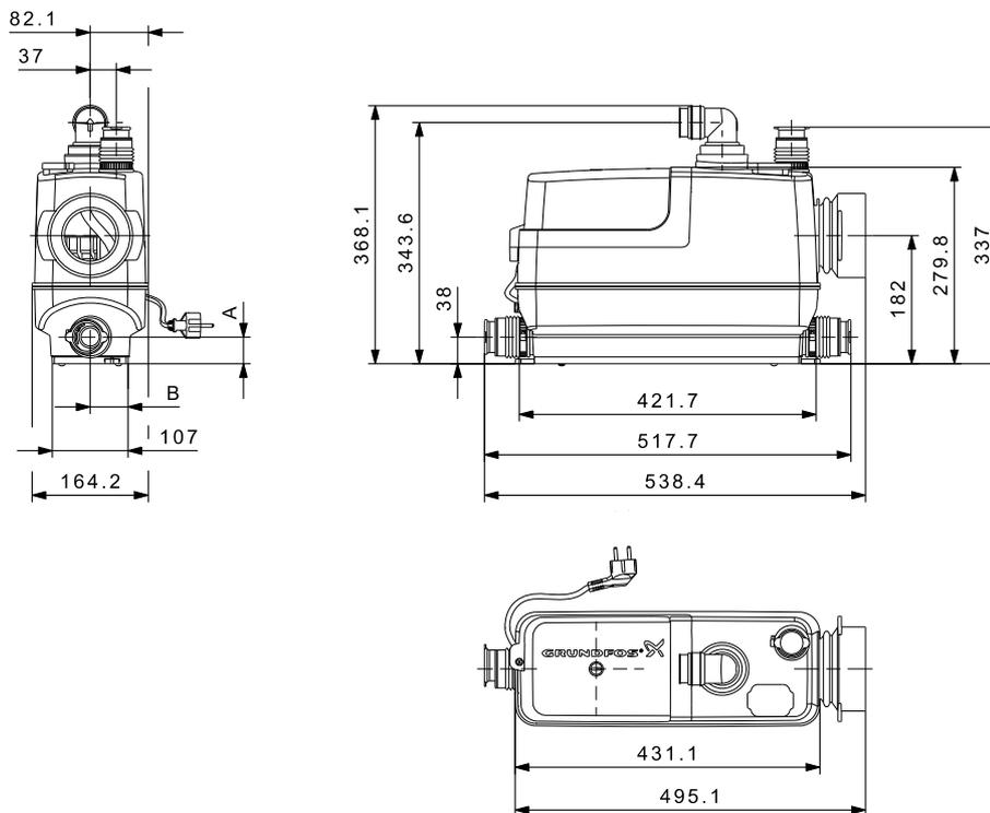
Fig. 27 Dimensions, Sololift2 CWC-3
