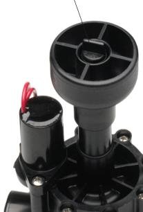
The external bleed allows perfect manual operation of the valve without electrically charging the solenoid. With the ability of users to bleed the valve to atmosphere, pressure is relieved and the valve can effectively open and close. System flushing can also be accomplished using the external bleed with debris and other material being flushed out of the port.
